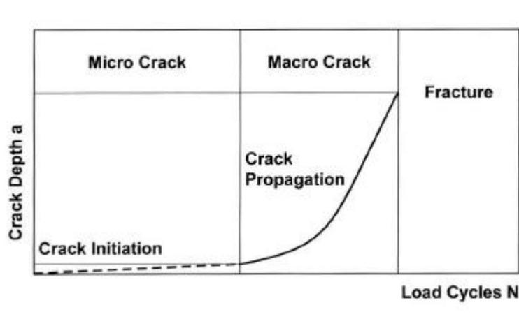
**Figure 7.** Illustration of crack propagation in hydro-electric turbine blading (Grein, 1998).
