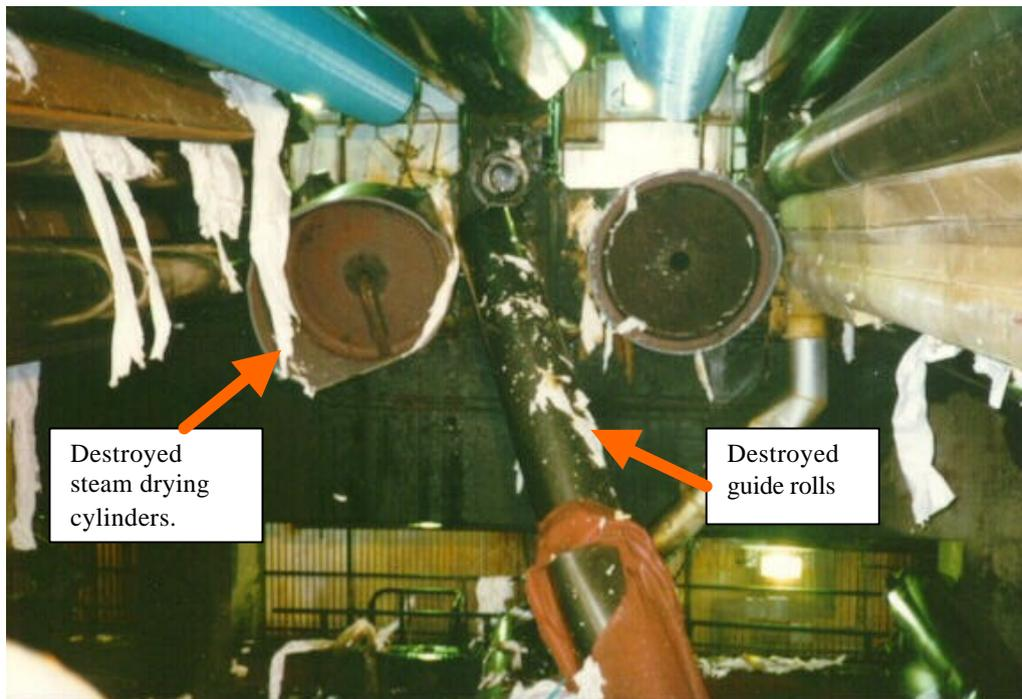
**Figure 10. Catastrophic failure of part of a large paper machine's drying section.**
